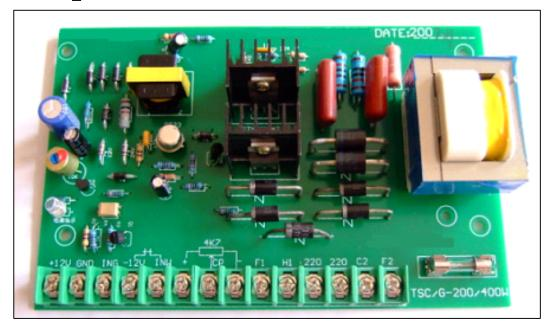
Thanks for using our factory TSC/G-200/400W DC motor control Board made in china.
